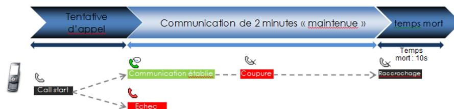
FIGURE 3 . PROTOCOLE DE MESURE QoS VOIX
